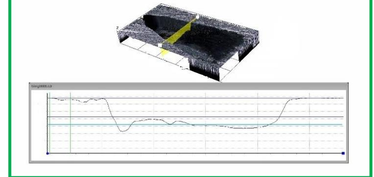
Microscopical analysis pointed out that recast layer in the diffuser can be avoided by performing a double scan in the diffuser floor area.
