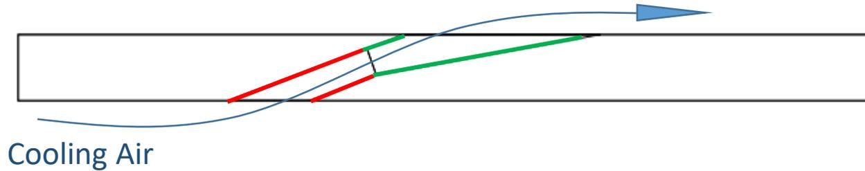
The use of holes with variable section (*shaped holes*) allows to increase the cooling efficiency of the combustion chamber.
