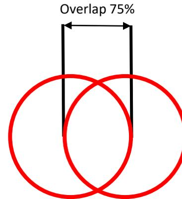
**Test 1: Reduced feedrate** while machining the diffuser floor (Overlap 75%).
