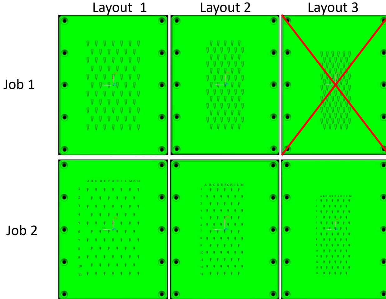
The extremely dense holes layouts can cause serious deformation of the plates during laser processing.
