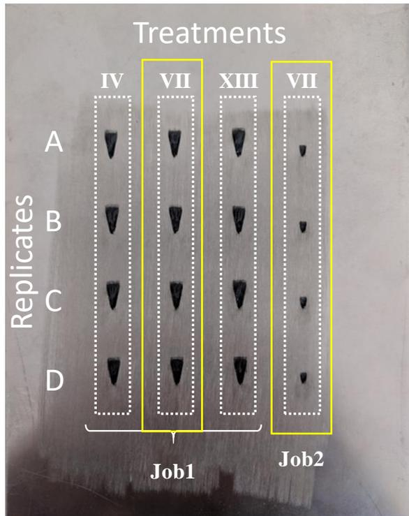
In previous thesis work, four sets of shaped holes were produced with the laser parameters assets (*treatments*) that had returned compliant results in terms of both geometrical and metallurgical characteristics, to be scanned by X-Ray Tomography.
