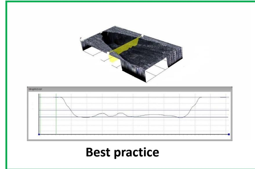
Based on results achieved for Job 1, laser beam pathway was modified also for Job 2, involving a counterclockwise movement starting from the bottom without double scan (since the diffuser of Job2 has no slope), so the drilling time per single hole is always the same.
