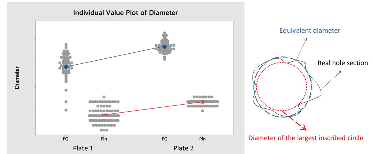
The mean difference detected through the pneumatic gauge and the pin gauge is almost the same.
